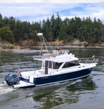
Performance, versatility, and comfort are central to the design of the Cutwater C-32 Command Bridge. The advanced double-stepped, deep-V hull combines speed, efficiency and superior stability. Our Laminar Flow Interrupters allow for smooth, positive cornering. Roll the throttles forward and you'll feel the powerful twin, counter-rotating 300 HP Yamaha outboards propel the C-32 CB to remarkable speeds.
